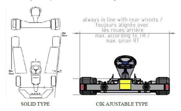
The two adjustable outer parts of the CIK homologated rear wheel protection must have a colour that is clearly different from the main part of the rear wheel protection. This can be done by a dedicated sticker kit or by adding colour to the parts during production. (01/01/2024)
