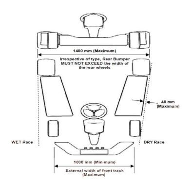
In dry configuration a plane joining the outer edge of the front and rear wheels shall be no further than 40mm from the side pod.
