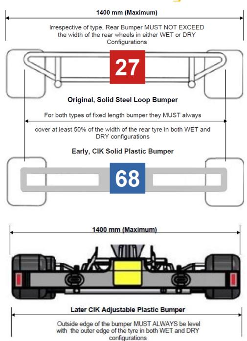
The two adjustable outer parts of the bumper should have a colour sticker, in a contrasting colour to the actual bumper. This should be visible from both the side and rear of the kart.
